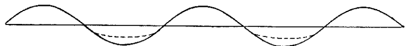
Fig. 21. The response of the ear-drum to a simple sound. The unsymmetrical nature of the human ear results in parts of the simple harmonic curve, which is drawn thick, being replaced by those shown by broken lines.
